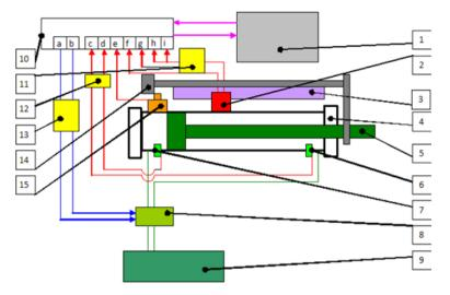
Figure 4 Hydraulic axis with mechatronic (hydronic) translation Components: 1. Computer PC, 2-3. Position transducer, 4-5. Hydraulic actuator, 6-7. Pressure transducer, 8. Proportional distributor, 9. Hydraulic power source, 10. Data acquisition card, 11. Position conversion circuit, 12. Pressure conversion circuit.
