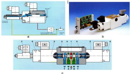
Figure. 3 a. Proportional distributor REXROTH, b. Picture distributor and control system, c. Constructive elements,
